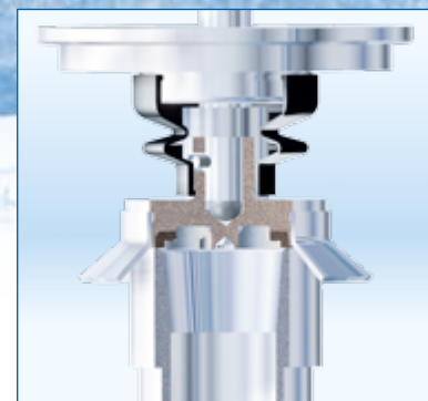
Optional EPDM bellows seal protects the stem from corrosion and sticking; soft sealing plug ensures reliable tight sealing; standard on SAFE heating valves SAFE Fig. 903
