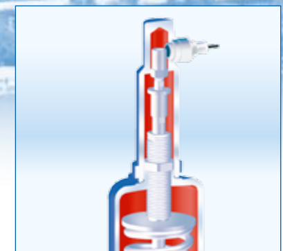
Integrated sensorics, proximity switch; used to return the feedback signal to the control room
